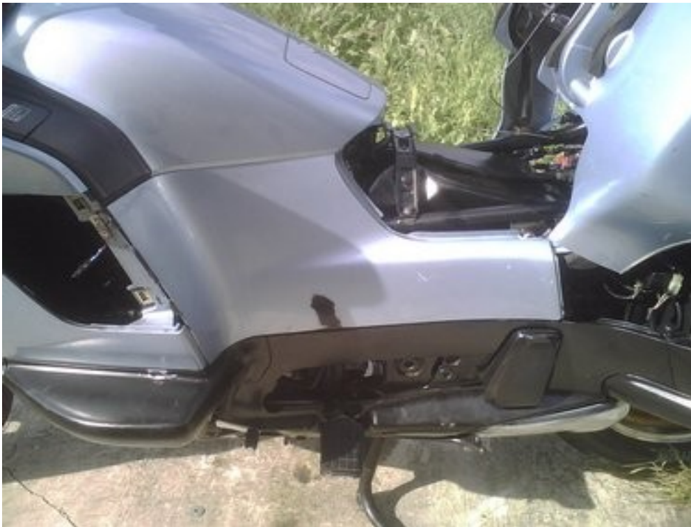
fit the left upper side cover I found it easy to leave the trunk open so you can push in the rear boss and leave of the step cover so you can get at the front lower boss
