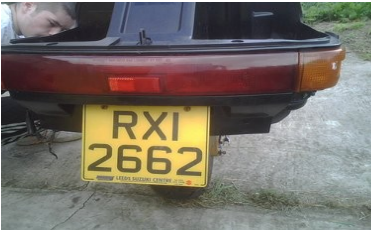
fit rear light and numberplate panel connect indicators and run trunk cable along frame and connect to loom
