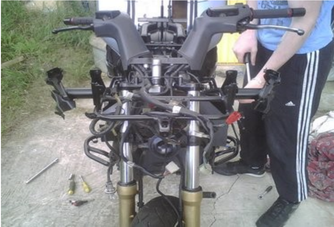
fit and bolt the fairing frame as well as the left and right air plates
