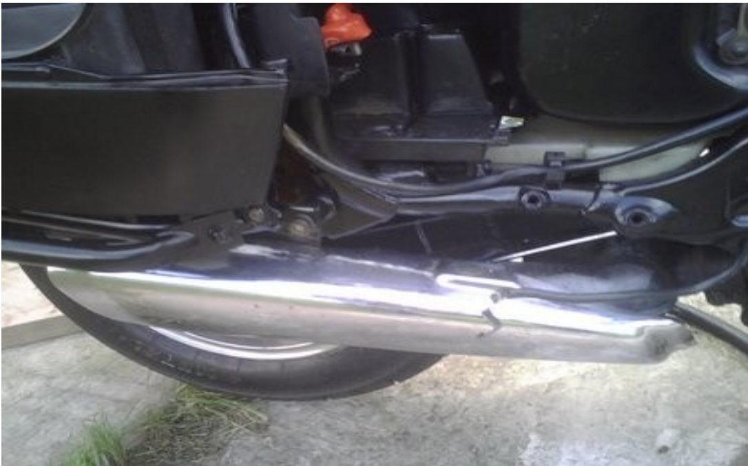
fit and bolt on the muffler connecting it to the rear down pipe
