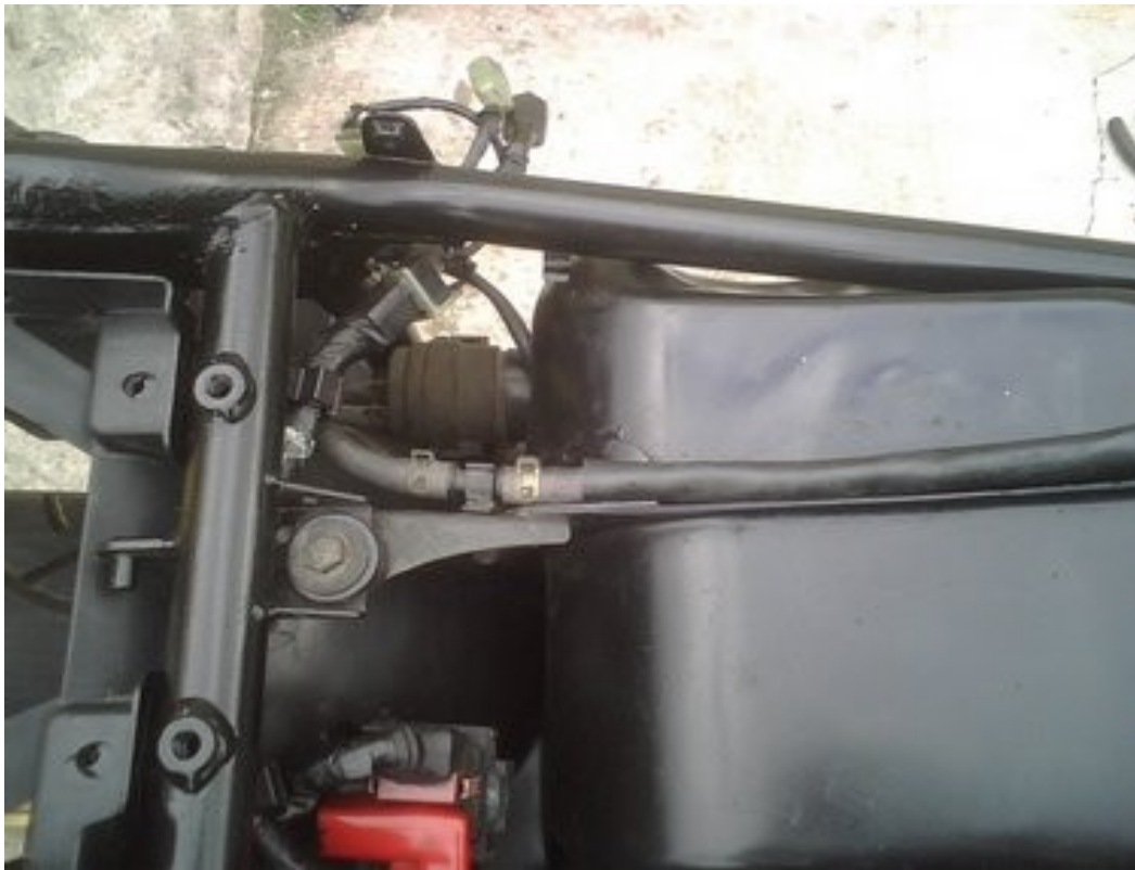
clip the fuel pipe to the bracket as seen the push pipe under clip further up
