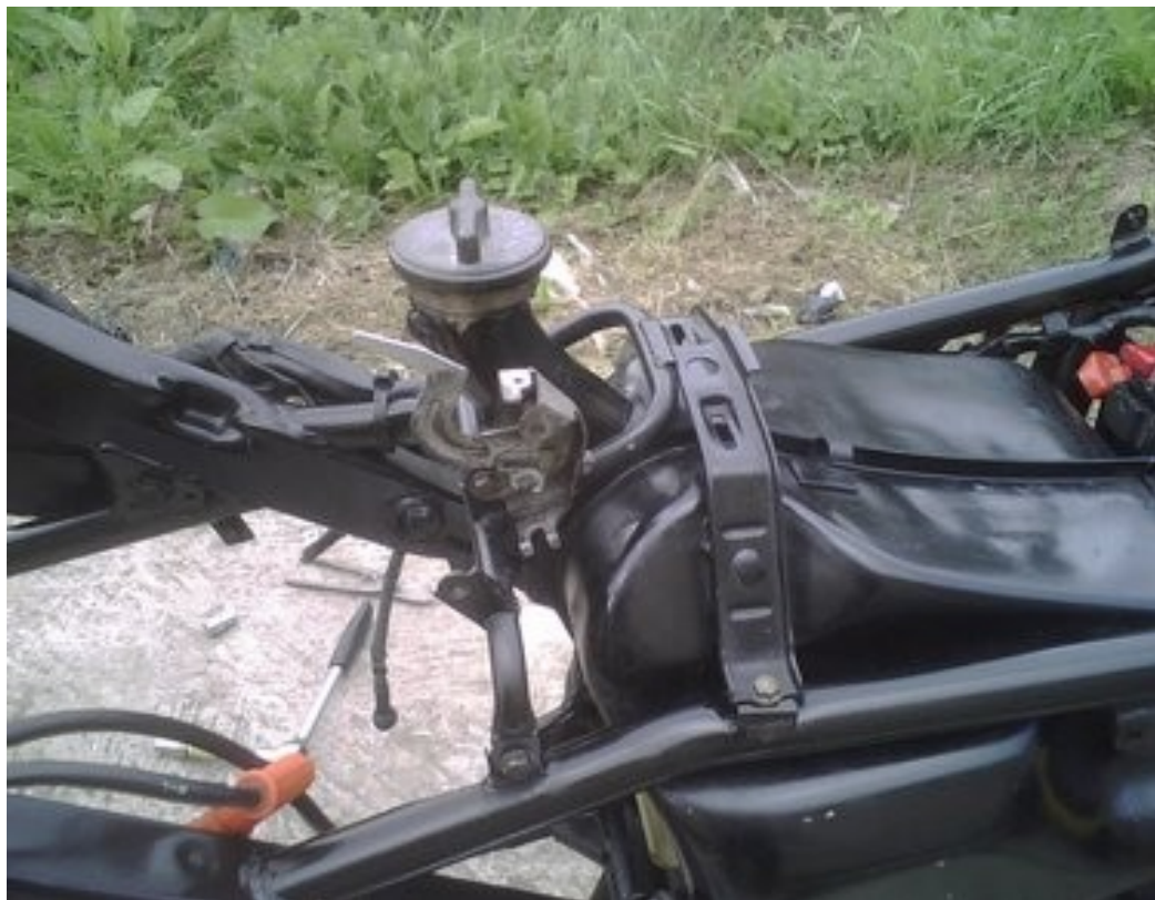
bolt on seat frame this was a mistake as it had to come off to get the plastic plates and heat shield on
