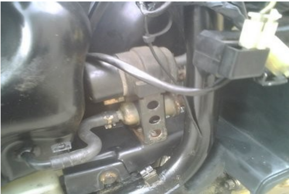
fuel pump and filter connect the pipes and connector
