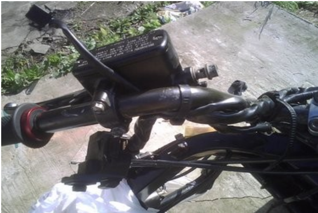
fit the clutch master cylinder and left grip and combination switch connect up the handlebar wiring check in the manual how the wiring routes around the handlebars tie in place with electrical ties
