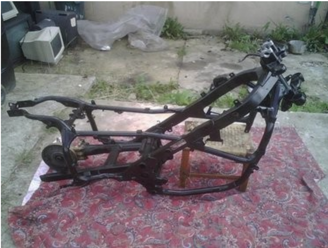
Frame from the left all nice and clean no rust
