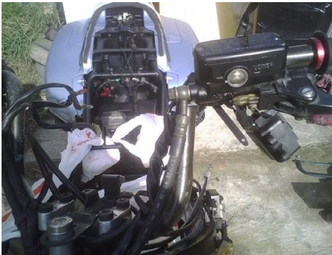
connect up the clutch pipe and run down the frame check manual for route
