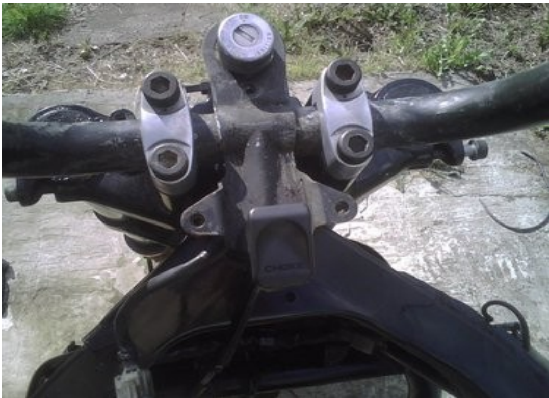
make sure the dots on the top clamps face forwards
