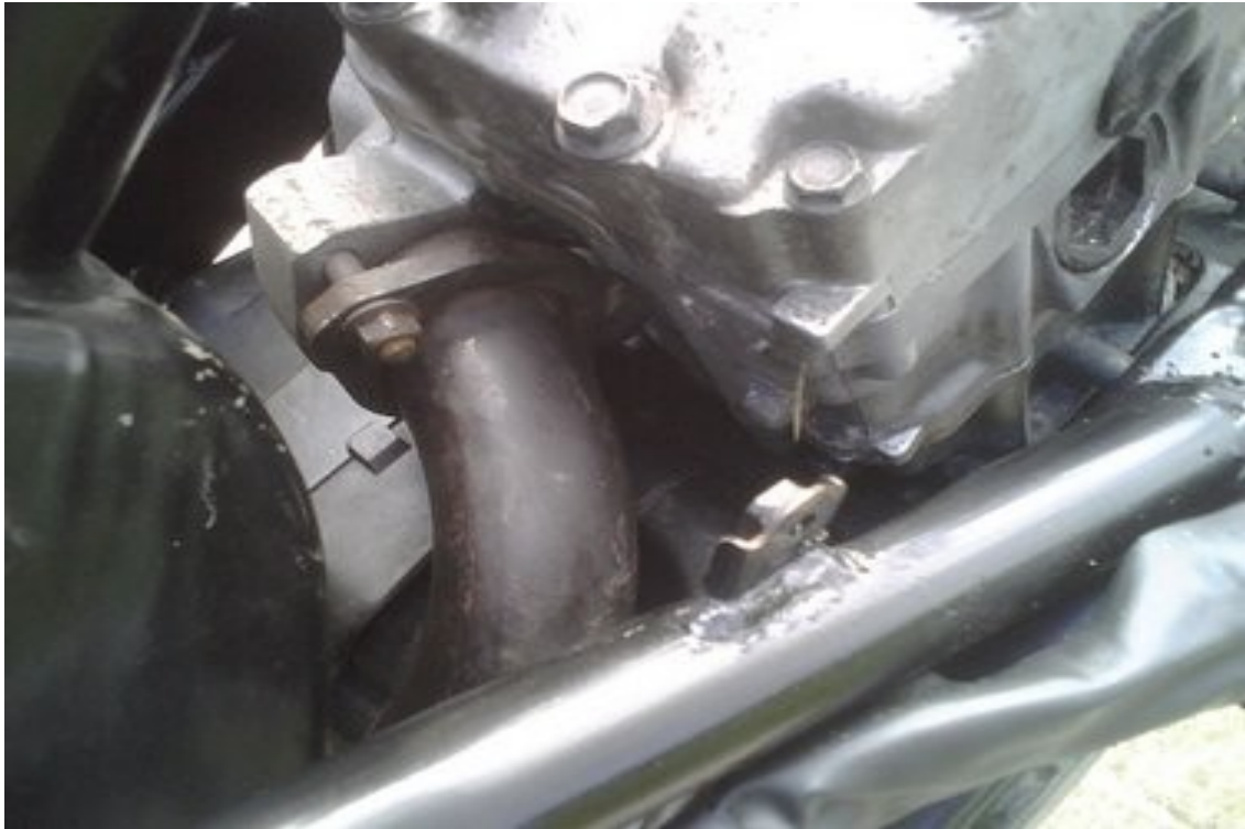
fit and bolt on the rear exhaust downpipe
