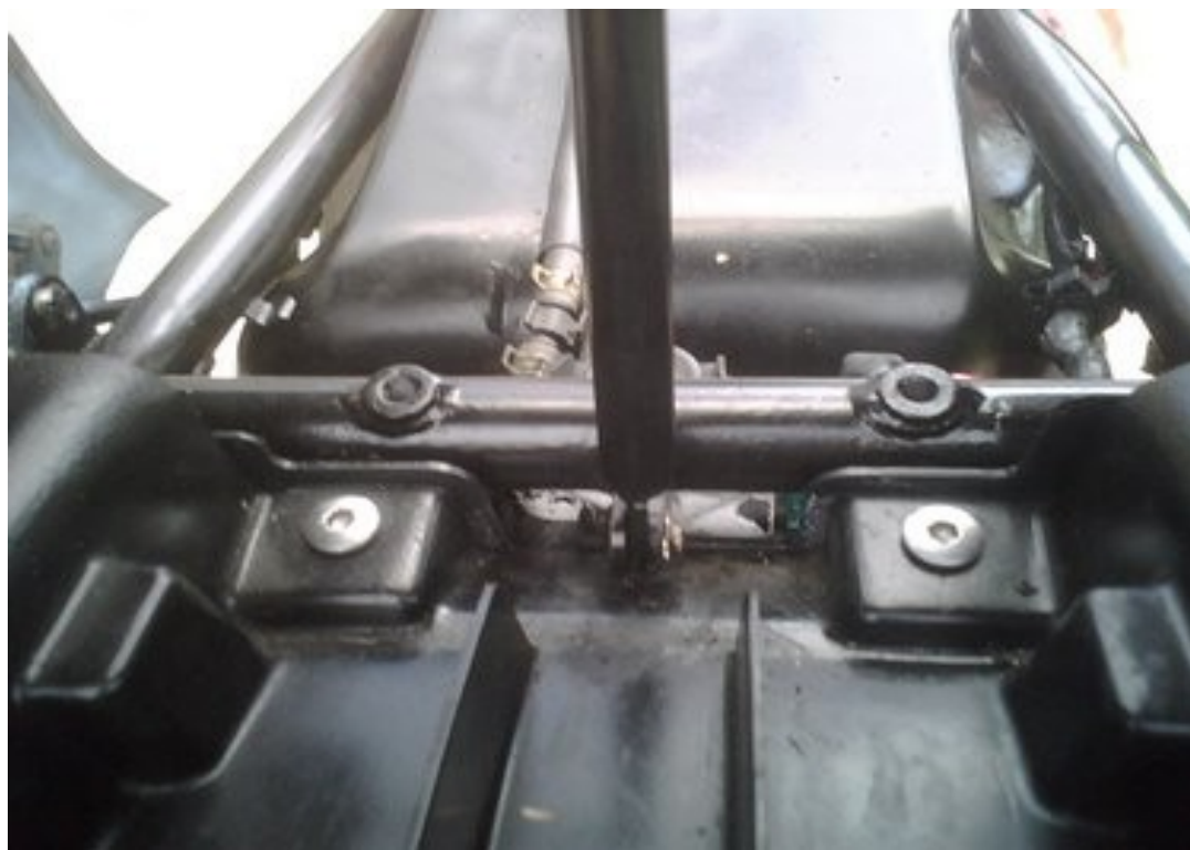
fit the bottom of the trunk lid gas shock found it easier to do it this way as the shock had opened up so connecting it to the top first you can the push the shock up so you can get it on the bottom peg found action was a little stiff so open and close a few times to get it working properly
