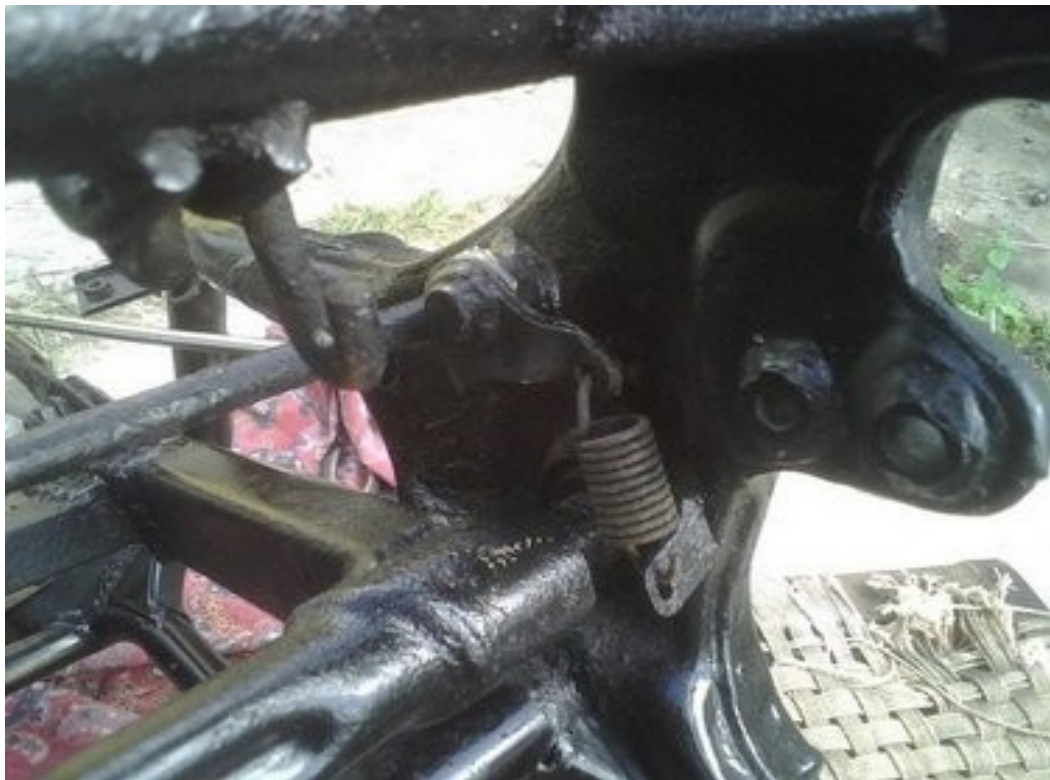
Brake mechanism fitted the bike is upside down at this point
