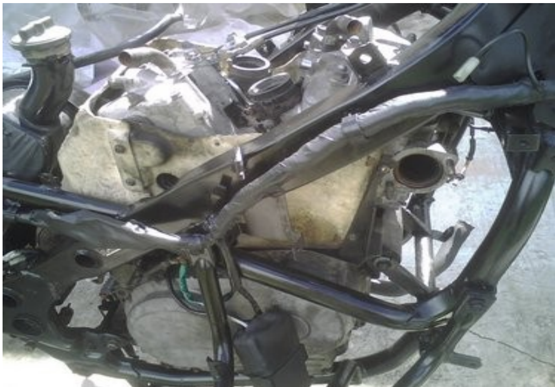
fit the right front side heat shield notice the broken rad shroud on the front of the heat shield
