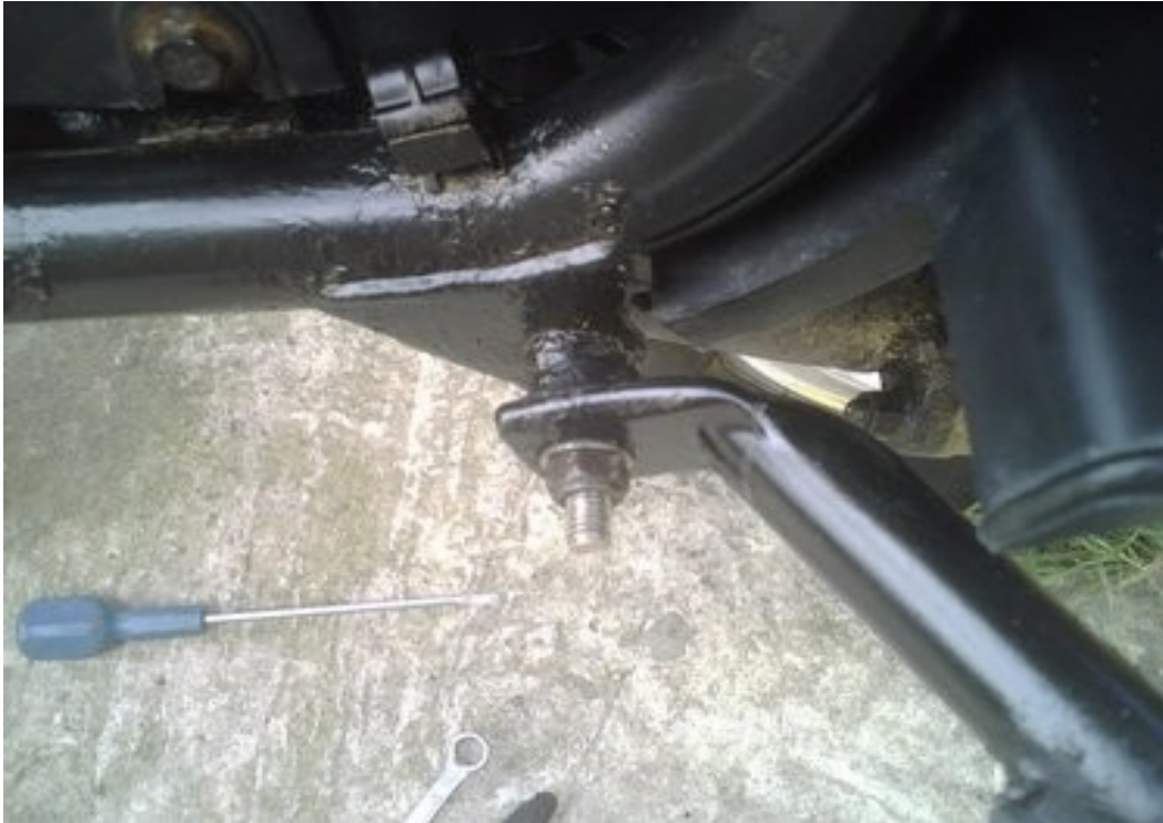
bottom left trunk frame bolt this one also broke so I drilled it out at 8mm and fit an 8x70mm bolt straight through the frame bracket and fixed with a washer and nyloc
