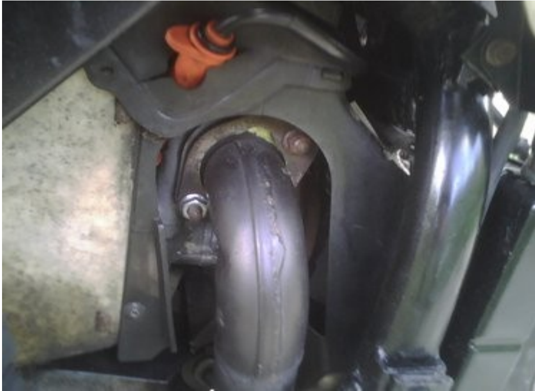
fit the lower front exhaust pipe to the muffler then fit the front upper exhaust pipe and bolt up see how the rubber mat holds my rad shroud in place
