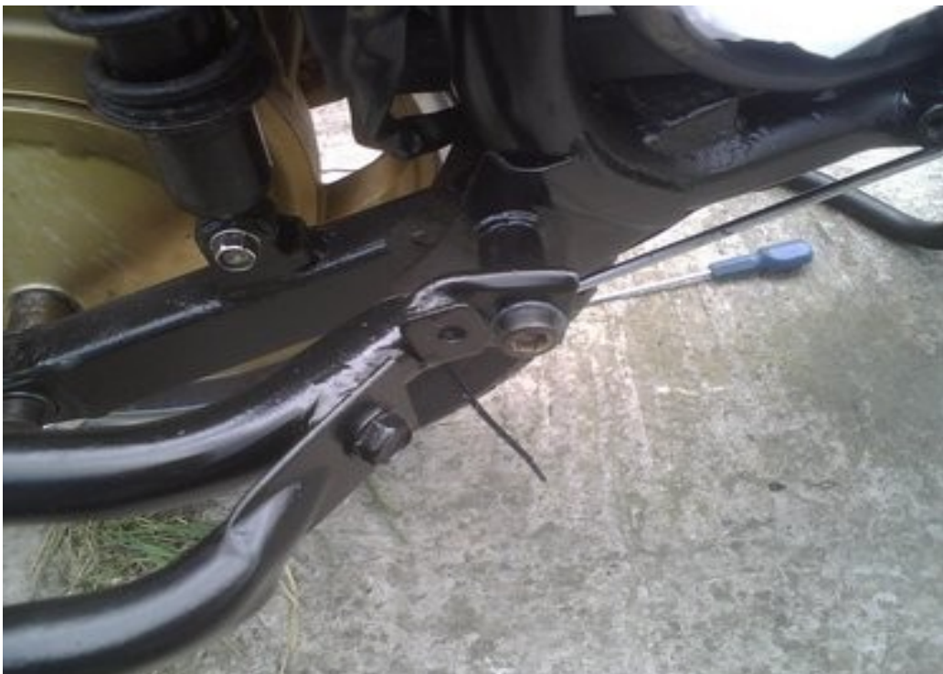
bottom left trunk frame bolt this one also broke so I drilled it out at 8mm and fit an 8x70mm bolt straight through the frame bracket and fixed with a washer and nyloc
